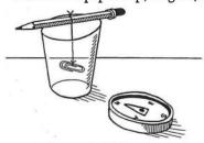
Here's how: First, your youngster will need to make one end of the paper clip magnetic by rubbing it along the magnet about two dozen times (rub in the same direction each time). To
