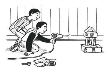
To test his building's strength, he can stand a few feet away and blow on it with a hair dryer set on low (to mimic wind). Does his building topple over, or does it just scoot along the floor? If the "wind" blows it down, suggest that he redesign and retest it. He'll figure out that a wide base and strong vertical supports affect how well a building can withstand wind.
